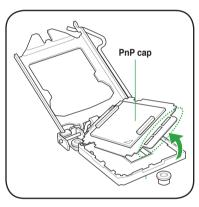
Position the CPU over the socket, ensuring that the gold triangle is on the bottom-left corner of the socket, and then fit the socket alignment keys into the CPU notches.
